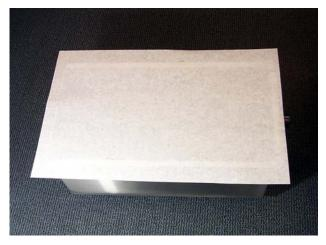
5. Position the hold-down ring over the filter paper and lower the ring into the pan, allowing the paper to fold up around the ring as it is pushed to the bottom of the pan.
