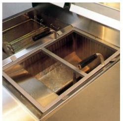
5. After the oil is filtered, close the drain valve and allow the fryer to refill. When bubbles appear in the oil, allow the filter to run 10 to 12 seconds longer to clear the lines and prevent shortening from hardening in them, then PUSH the filter handle to the OFF position (arrow).
