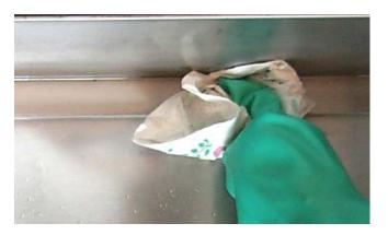
4. Lay one sheet of filter paper over the top of the filter pan, overlapping on all sides.
