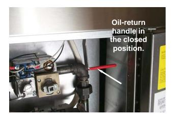
5. Remove the Power Shower and allow it to drain. Ensure the drain valve is fully closed (arrow). Turn the fryer ON and allow the oil to reach setpoint.
